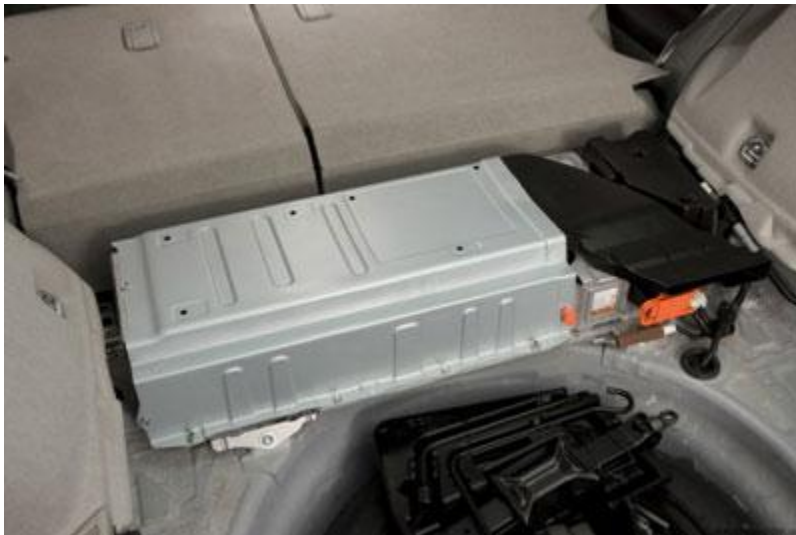
Nickel metal hydride battery pack in 2010 Toyota Prius.
