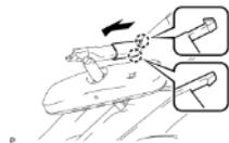
(1) Disengage the 2 claws and slide the inner rear view mirror cover as shown in the illustration.
