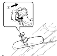
(b) Remove the inner rear view mirror as shown in the illustration.
