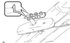
(2) Disengage the 6 claws and remove the inner rear view mirror cover.
