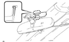
(2) Disengage the 2 claws and remove the inner rear view mirror cover.
