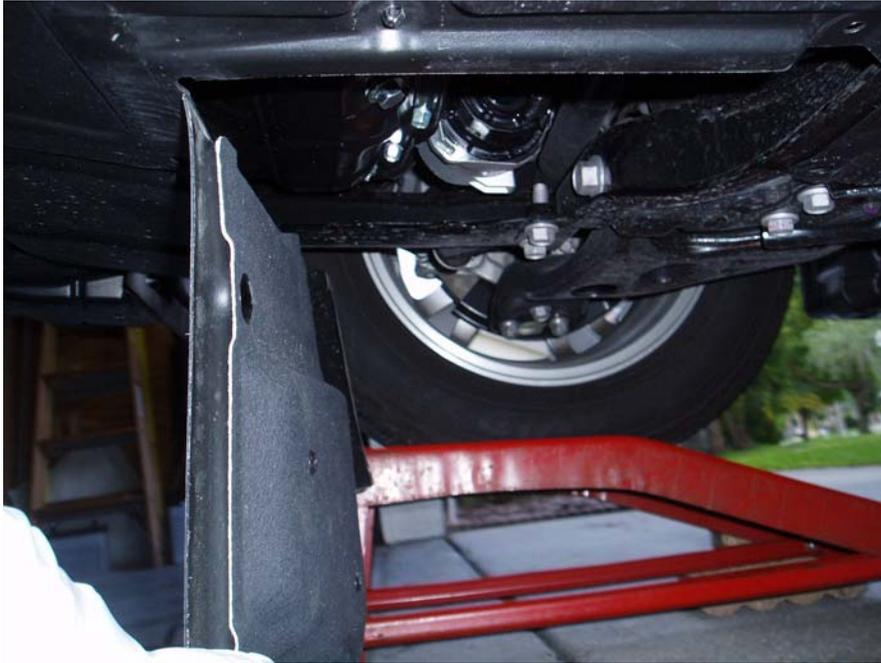
10. Re check to make sure the housing is tight (snug do not over torque) and the Drip Pan Drain Plug / Bolt is secure.
